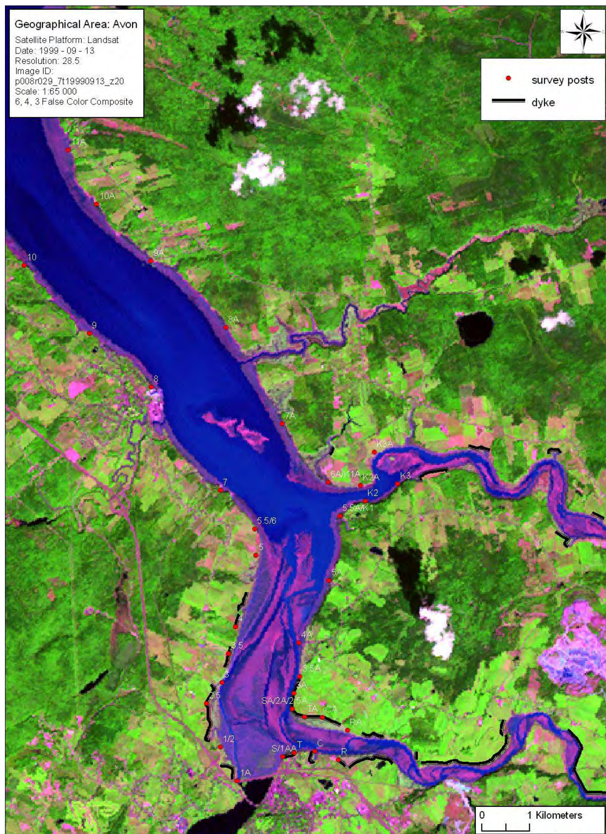
Figure 4.29: Landsat 7 bands 6,4,3 false color composite illustrating position of main channels and intertidal bedforms at low spring tide. Note position of sand wave near Hantsport.
